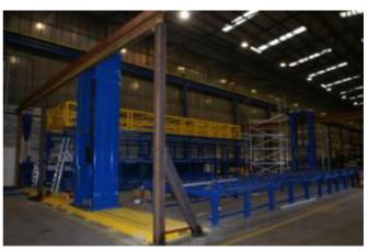
To improve manufacturing output of containerised diesel generators at the Larne plant Lindhurst Innovation Engineers manufactured a series of bespoke jigs & manipulators to assist in the manufacturing process of the generator housing units (10 to 45 feet in length). Within one month of commissioning the capacity doubled
